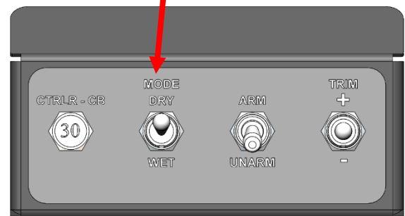
TLEG Panel Located in Cockpit
