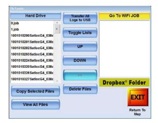
To transfer files from the hard drive to your Dropbox account select a file in the Hard Drive file list then press the arrow button.
