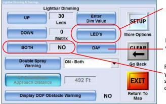
Press to switch between LEDs and Matrix; what shows on this button determines what you adjust with the UP/DOWN, Enter Dim Value, and Both buttons
