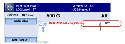
3. Press the **POLYS** button repeatedly to cycle through multiple log files on the map.
